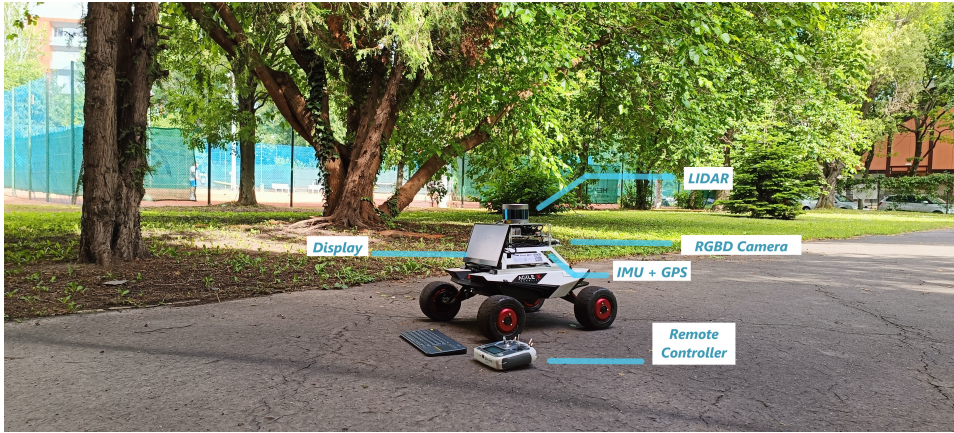
Figure 1. Pomona: a ROS 1-based multi-sensor robotic platform used in our experiments. The system integrates a Velodyne VLP-16 LiDAR, an Intel RealSense D435 RGB-D camera, an Xsens IMU, and a GNSS receiver.
