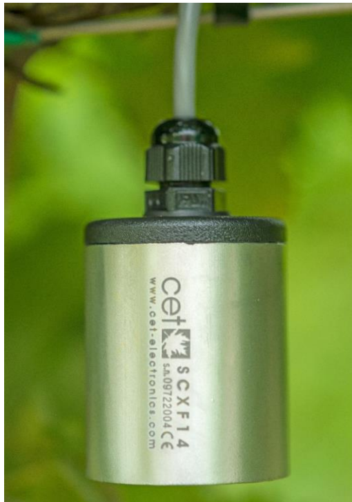
22. Figure Air temperature and humidity intracanopy sensor
