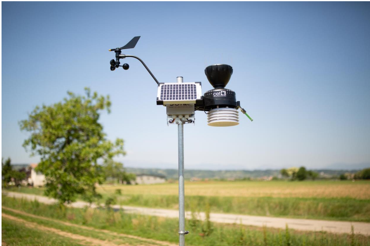
17. Figure Weather station with multiple sensors in the field
