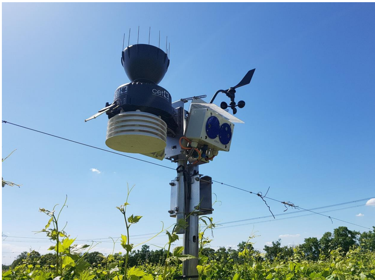
26. Figure Weather station equipped with stereo camera
