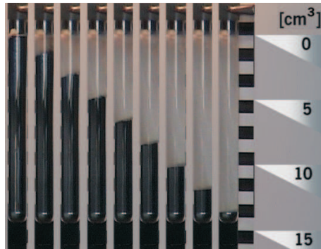
Figure 1: Crystallization of Sodium Acetate in a test-tube.
