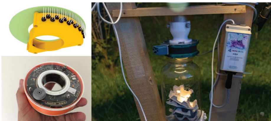
Figure 2. Zoolog ring and data collector, and as it is attached to the Jermy trap. Source: zoolog.hu (2020), image taken by István Gyarmathy (2020)
