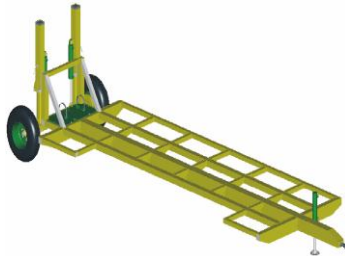
Fig. 1 Virtual model of the designed tractor trailer aimed for transport of seeding machines
