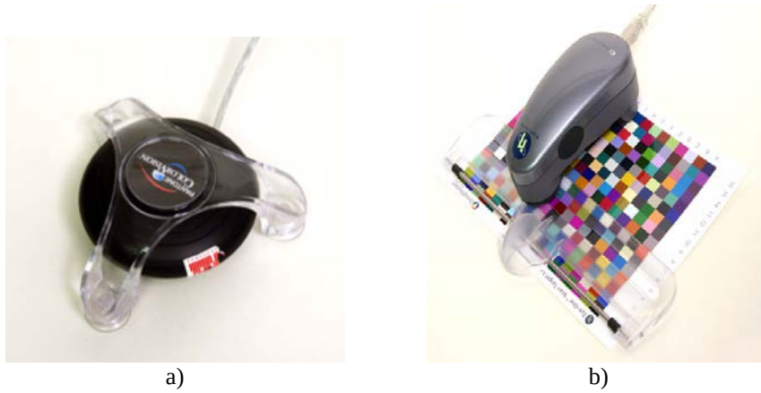
Figure 3: Equipment for colour measurement. a) - Panton Spyder fotolorimetr and b) - Gretag Makheth Eye One spectrophotometer with colour target.
